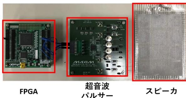
Fig.6 Equipment used for speaker drive circuit
